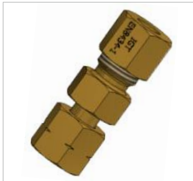
Nut entry 8 mm compression fitting Exits G1/4-19LH female Reference A900-236
